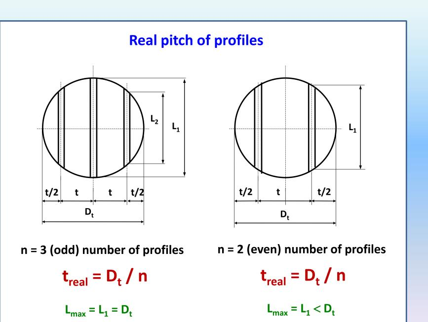
In our example is n = 2 profiles, i = 1 (only 2 symmetric profiles) so that we can use the above calculated result  $L_1 = 909$  mm.
