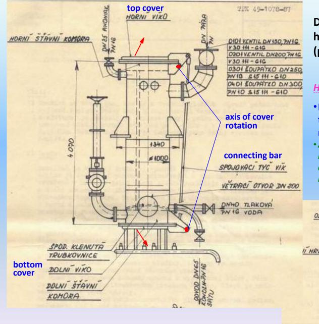
Drawing of the actual tube heater with basic dimensions (producer ZVU Hradec Králové)
